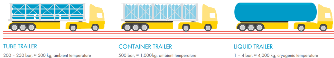
Exhibit 5: Transporting & storing hydrogen in various states
